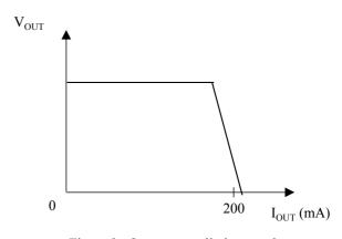
Figure 3. Over current limit control
