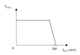
Figure 3. Over current limit control
