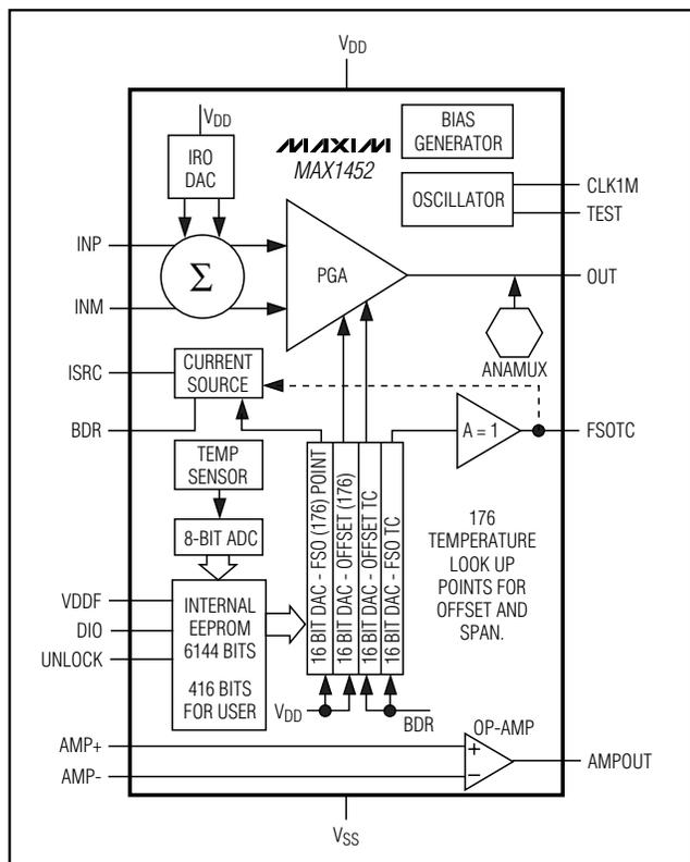
Figure 1. Functional Diagram
