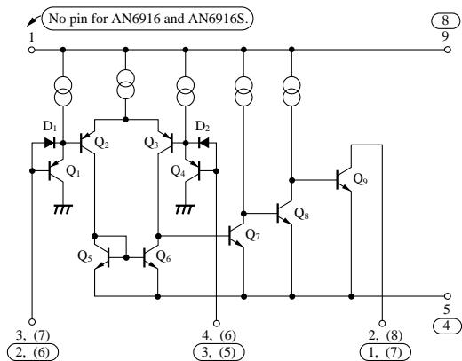
Note 1) The No. in ( ) are pin No. of AN6916 and AN6916S.
