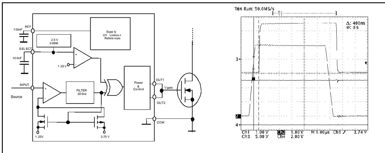
In applications requiring electrical isolation, the SELECT pin is designed especially for biasing a pulse transformer. Then, the quiescent level at INPUT pin is shifted to 2.5V and there is a differential threshold of +1.25V at switch-on and -1.25V at switch off.
