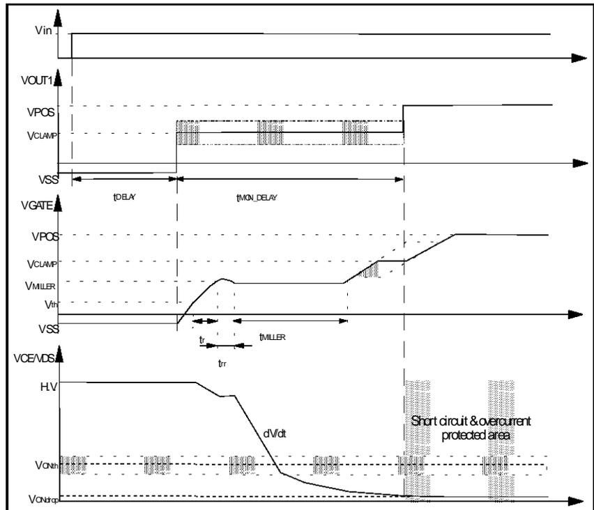
The relationships between the gate clamped voltage and a resistive divider (from REF pin) is:
