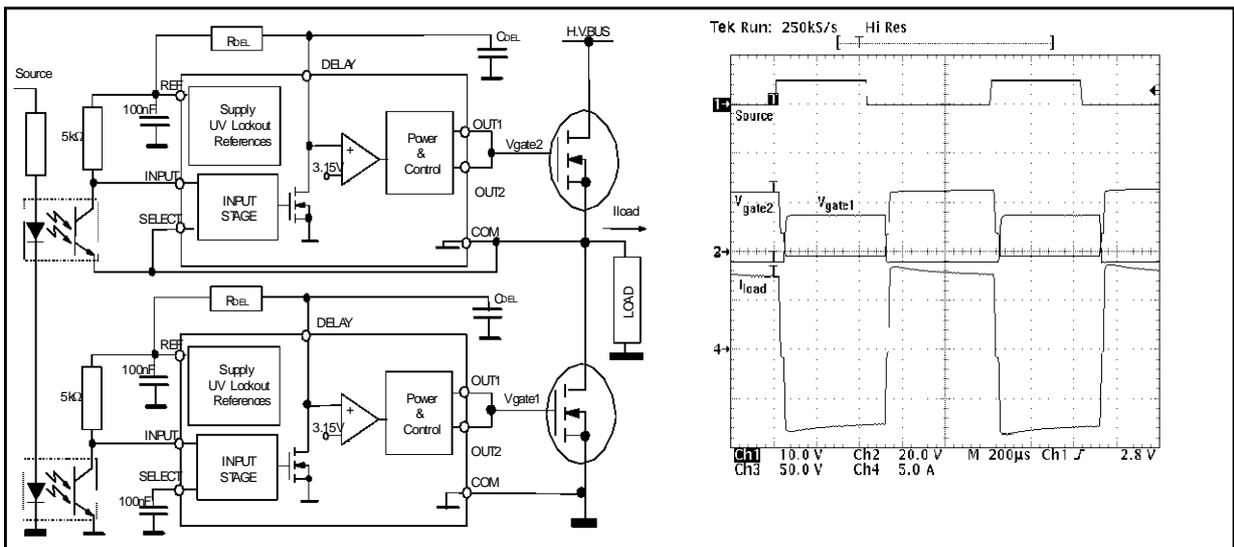
The relationship between the RC parts value and the internal timing circuitry is:
