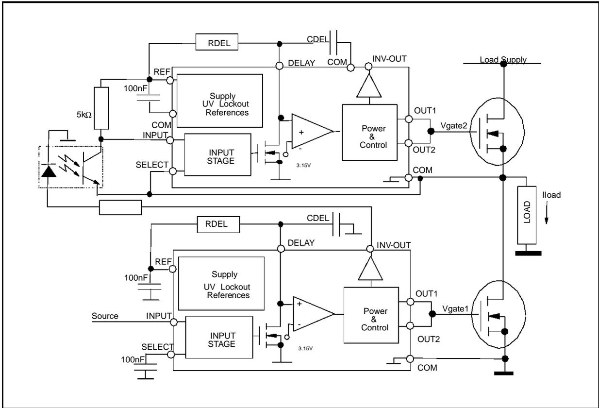
**Aligning the switching edges**
