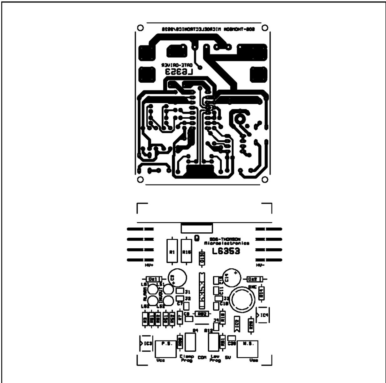
Figure 17. TEST-circuit schematic.
