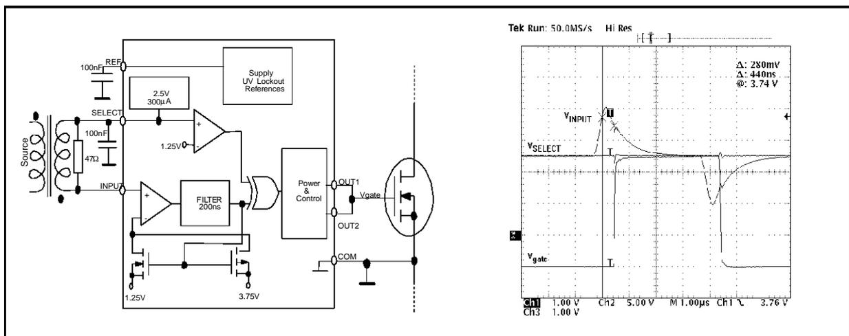
A cheap way to get the electrical isolation resorts to an optocoupler. In this case, the built-in 5V at VREF pin can be used to bias the optocoupler and, of course, the SELECT pin allows to manage the phase.
