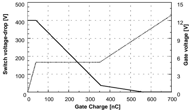
To reach the gate voltage needed for a full conduction of the switch, a certain amount of charge (depending both on the switch and the application) must be stored into the gate capacitance. Since this is charged with a limited current source, the switch turn-on transition needs some time. This means that until transition is completed, the monitoring of the switch voltage drop must be blanked. The relationships between the blanking time and the RC cell (from REF pin) is:
