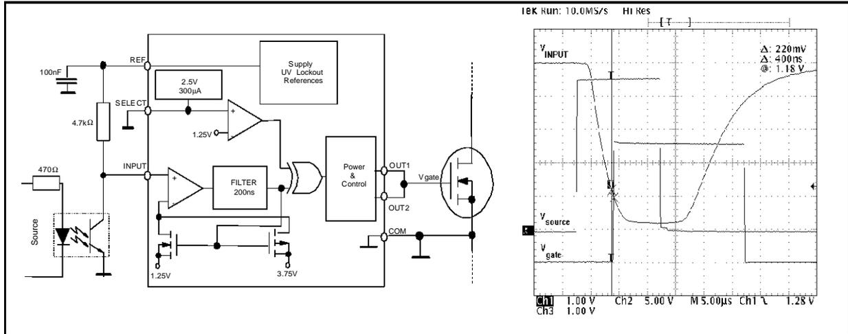
**Failure warning at the alarm output**
