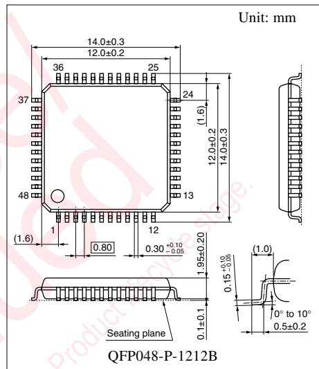
Note) The package of this product will be changed to lead-free type (QFP048-P-1212C). See the new package dimensions section later of this datasheet.
