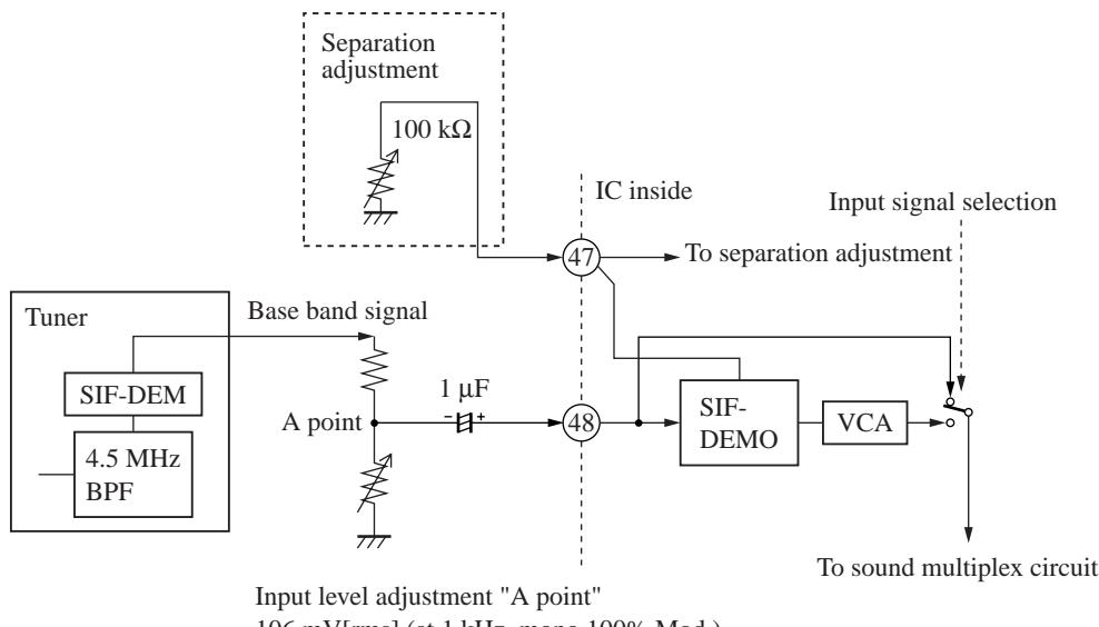
Note) Pin 47 must be open when separation is adjusted with the potentiometer of input level adjustment.
