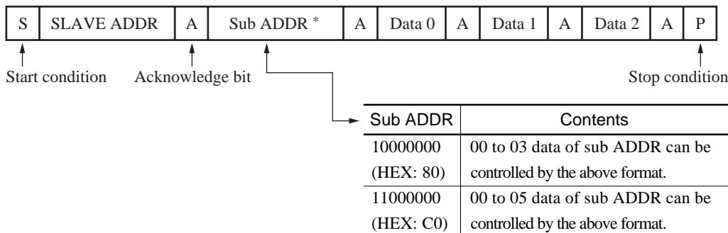
Once the data is inputted as shown above, the specified sub-address data is set to Data 0, one increment data to Data 1, further one increment data to Data 2. In this way, the plural data can be controlled at one time.
