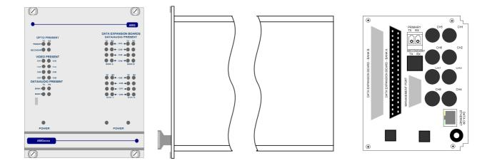
The **AMG4707AEG** is a rackmount data transmit unit designed to transmit and receive up to 8 data or audio signals plus full duplex 100BaseT Ethernet connectivity over two singlemode fibres. The 8 data/audio channel interfaces, whether RS232, RS422, RS485, 20mA, TTL, Contact Closure, Lonworks or Audio, are defined at manufacture by the addition of daughter boards fitted onto the Data Expansion Board A.
