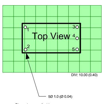
Dimensions mm (inch) Case Tolerance  $\pm 0.50$  ( $\pm 0.02$ ) Pin Diameter 1.0  $\pm 0.05$  (0.04  $\pm 0.002$ ) Pin Pitch Tolerance  $\pm 0.35$  ( $\pm 0.014$ )
