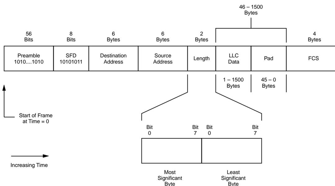
**Figure 34. IEEE 802.3 Frame And Length Field Transmission Order**
