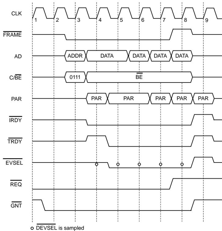
**Figure 15. Burst Write Transfer (EXTREQ = 1)**
