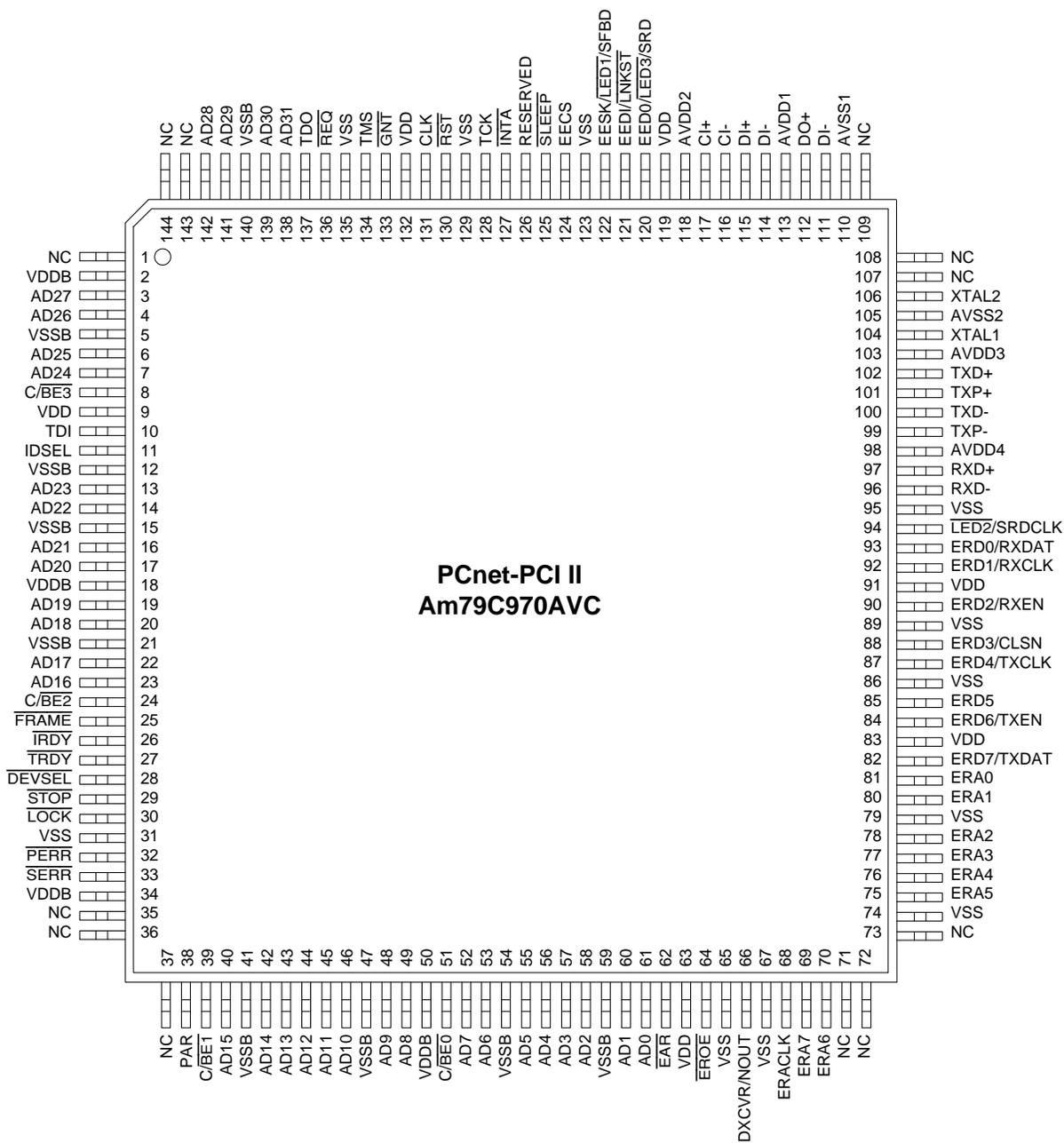
Pin 1 is marked for orientation.
