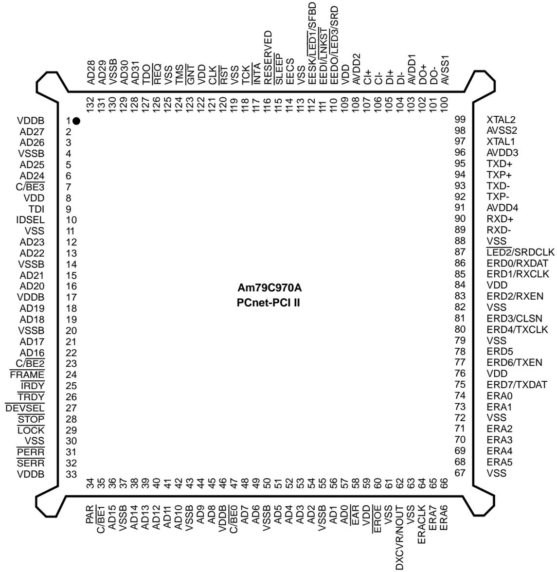
Pin 1 is marked for orientation
