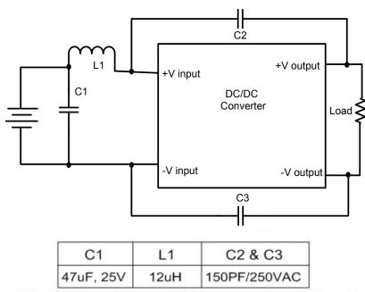
C2 & C3: Y5P Safety Standard Recognized Ceramic Capacitors foot distance 10mm
