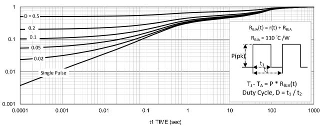
11. Normalized Thermal Transient Junction to Ambient
