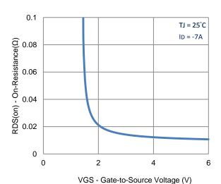
3. On-Resistance vs. Gate-to-Source Voltage
