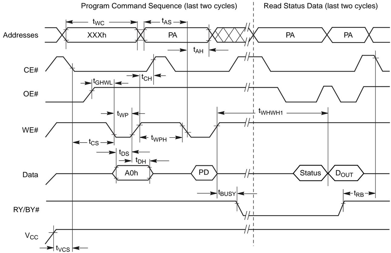
**Note:** PA = program address, PD = program data, D<sub>OUT</sub> is the true data at the program address.
