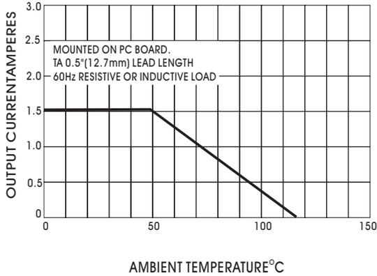
Fig. 1- DERATING CURVE FOR OUTPUT RECTIFIED CURRENT
