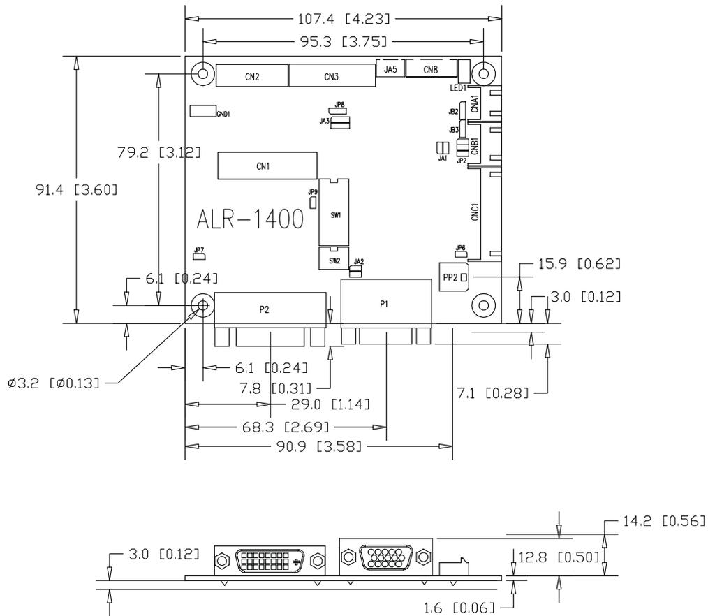
The maximum thickness of the controller is 15.8mm (measured from bottom of PCB to top of components, including any underside components & leads). We recommend clearances of:
