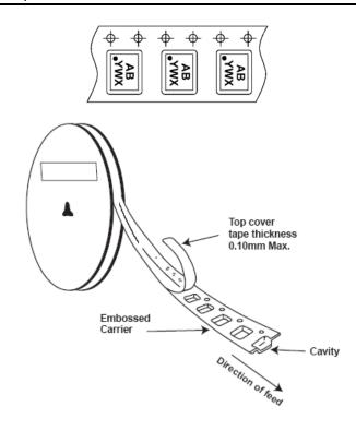
Notes: 9. The taping orientation of the other package type can be found on our website at http://www.diodes.com/datasheets/ap02007.pdf
