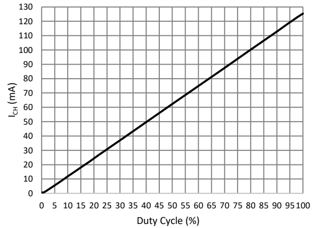
PWM to Analog Dimming Curve @ f_{PWMA} = 100\text{kHz} Channel Current vs. Duty Cycle
