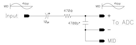
\*Note: Position capacitor as close to pins as possible. Film or high quality ceramic capacitor suggested.
