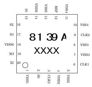
Package: 20-Pin QFN(Top View)
