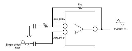
Figure 5. Non-Inverting Single-ended Input
