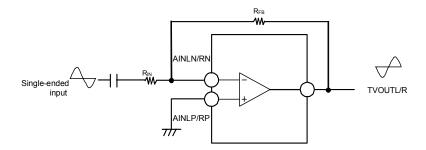
Figure 4. Inverting Single-ended Input
