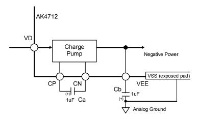
Figure 6. Negative Power Generate Circuit
