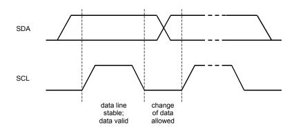
Figure 17. Bit Transfer on the I<sup>2</sup>C-bus
