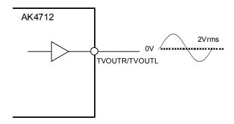
Figure 7. Audio Signal Output
