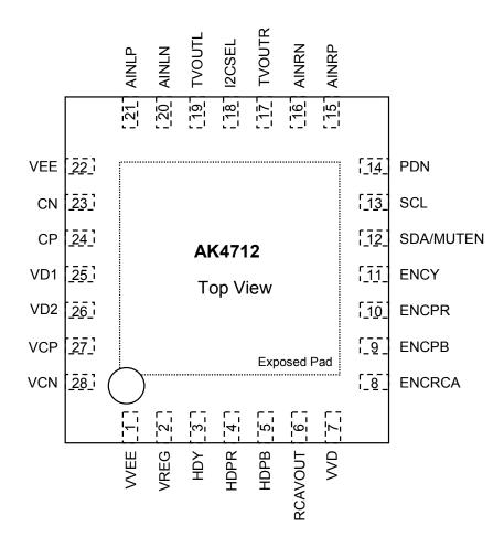
Note 1. The exposed pad on the bottom surface of the package must be connected to VSS.
