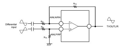
Figure 3. Full Differential Stereo Input
