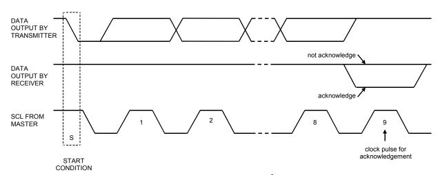
Figure 16. Acknowledge on the I<sup>2</sup>C-bus
