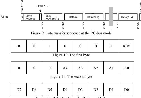
Figure 12. Byte structure after the second byte
