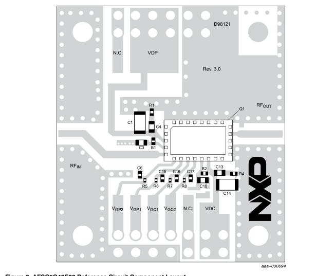
Figure 2. AFSC5G40E38 Reference Circuit Component Layout
