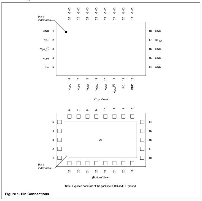
1.  $V_{DP2}$  and  $V_{DC2}$  are DC coupled internal to the package and must be powered by a single DC power supply.
