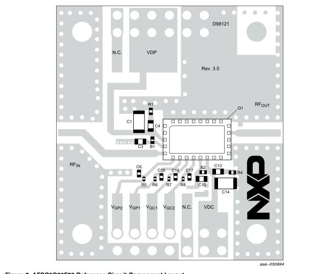
Figure 2. AFSC5G26F38 Reference Circuit Component Layout
