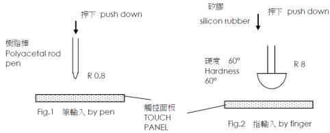
Notes area for pen notes life test is 10×9mm. Size of word is 7.5×6.75mm. Word is any A.B.C..... Word. Center of each word is changed at random on active area inside 5mm.
