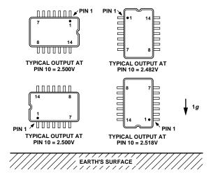
Figure 1. ADXL190 Response Due to Gravity
