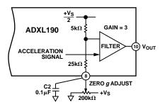
Figure 2. Optional Zero-g Adjust Circuit Detail
