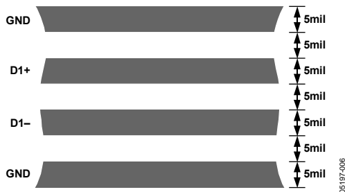
Figure 18. Arrangements of Signal Tracks
