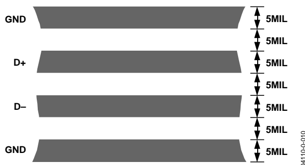
Figure 24. Typical Arrangement of Signal Tracks
