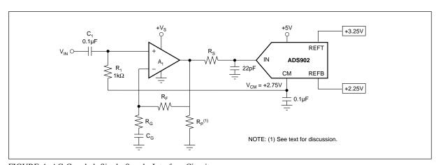
FIGURE 4. AC-Coupled, Single-Supply Interface Circuit.
