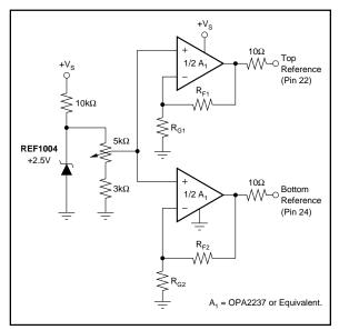
FIGURE 7. Precise Solution to Supply External Reference Voltages to the ADS902.
