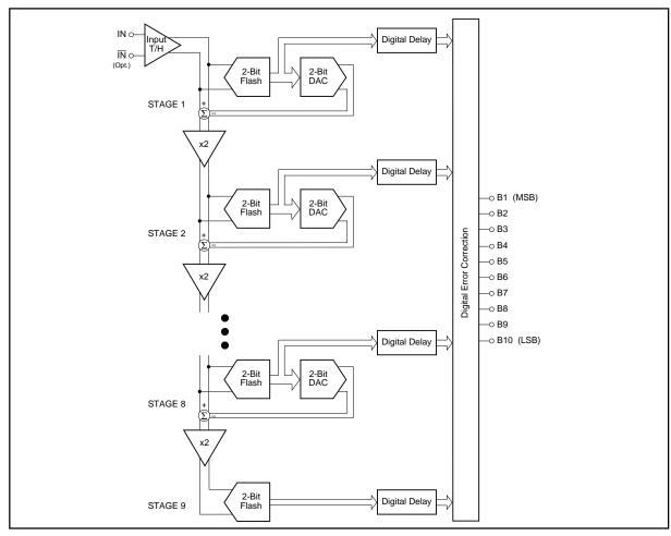
FIGURE 2. Pipeline A/D Architecture.
