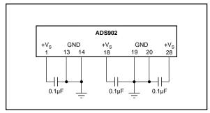
FIGURE 9. Recommended Bypassing for Analog Supply
