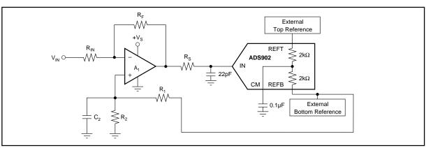
FIGURE 5. DC-Coupled, Single-Supply Interface Circuit.
