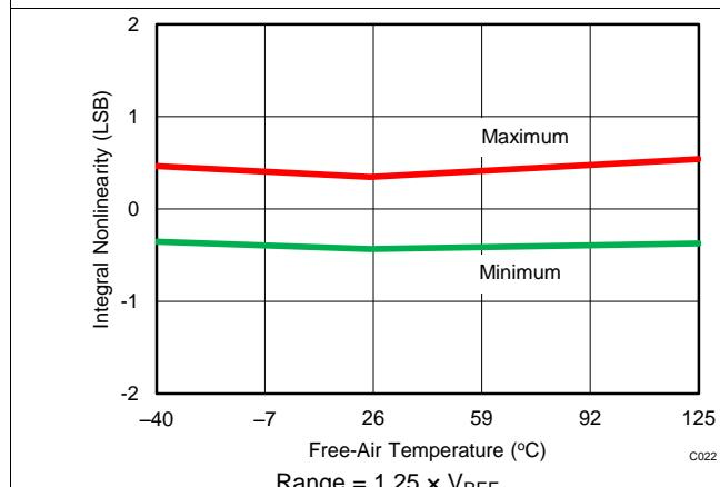
**Figure 22. INL vs Temperature ( $1.25 \times V_{\text{REF}}$ )**
