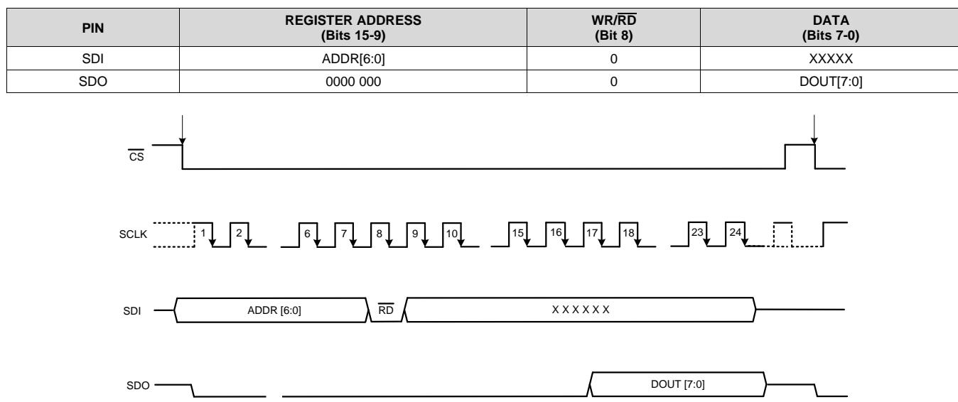
**Figure 89. Program Register Read Cycle Timing Diagram**
