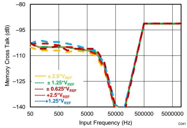
Figure 41. Memory Crosstalk vs Frequency
