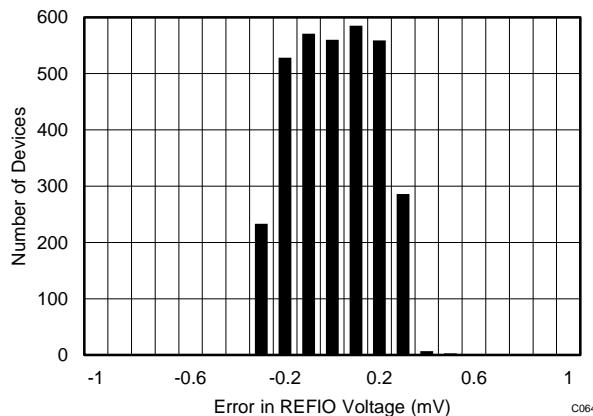
**Figure 58. Internal Reference Accuracy at Room Temperature Histogram**
