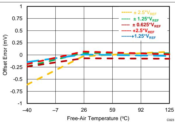
**Figure 23. Offset Error vs Temperature Across Input Ranges**
