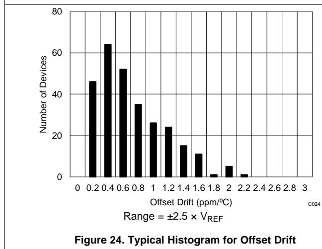
**Figure 24. Typical Histogram for Offset Drift**
