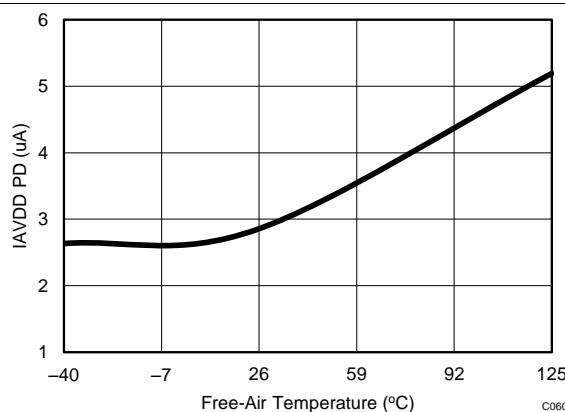
**Figure 50. AVDD Current vs Temperature
