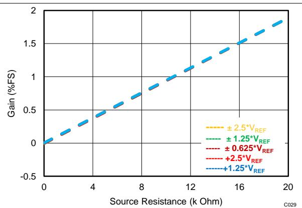
**Figure 29. Gain Error vs External Resistance ( $R_{\text{EXT}}$ )**
