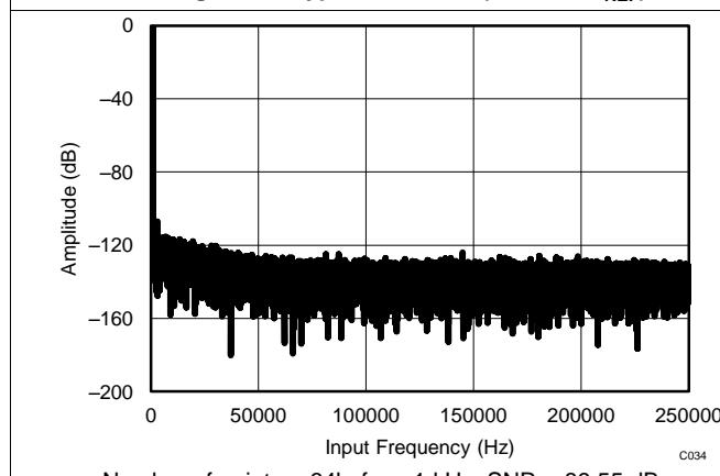
**Figure 34. Typical FFT Plot ( $1.25 \times V_{\text{REF}}$ )**
