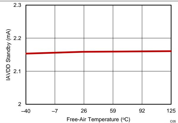
**Figure 49. AVDD Current vs Temperature (STANDBY)**
