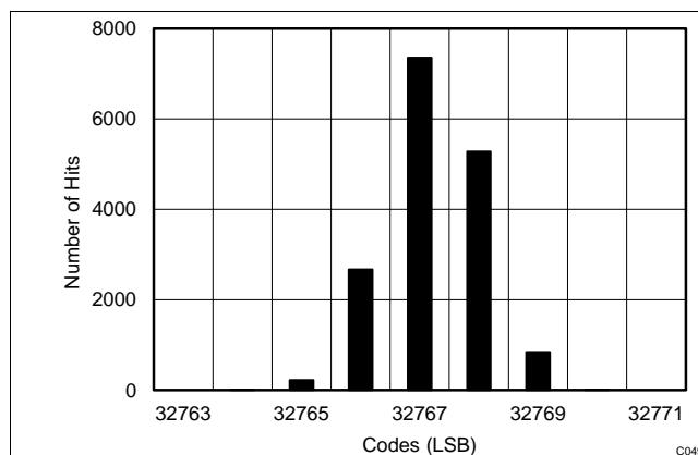
**Figure 65. DC Histogram for Mid-Scale Input (AUX Channel)**
