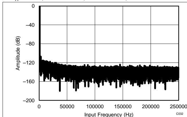
**Figure 32. Typical FFT Plot ( $\pm 0.625 \times V_{\text{REF}}$ )**
