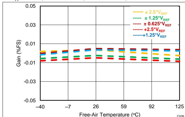
**Figure 26. Gain Error vs Temperature Across Input Ranges**
