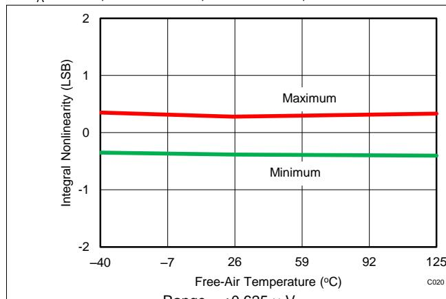
**Figure 20. INL vs Temperature ( $\pm 0.625 \times V_{\text{REF}}$ )**
