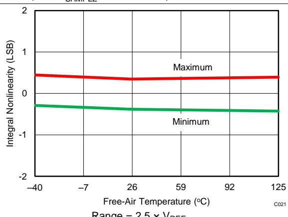
**Figure 21. INL vs Temperature ( $2.5 \times V_{\text{REF}}$ )**
