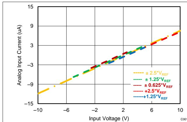
Figure 2. Input I-V Characteristic
