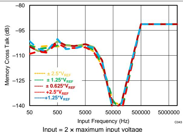
Figure 43. Memory Crosstalk vs Frequency for Overrange Inputs
