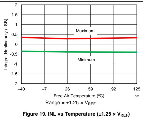
**Figure 19. INL vs Temperature ( $\pm 1.25 \times V_{\text{REF}}$ )**
