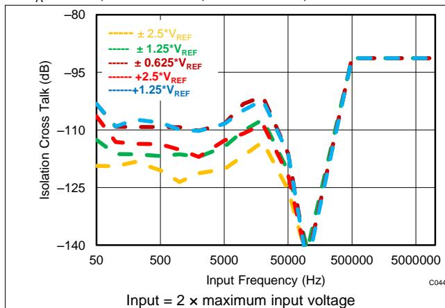
**Figure 44. Isolation Crosstalk vs Frequency for Overrange Inputs**
