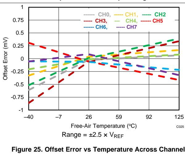
**Figure 25. Offset Error vs Temperature Across Channels**
