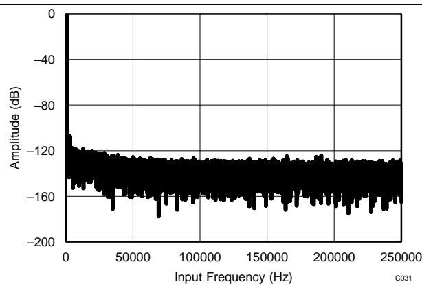
**Figure 31. Typical FFT Plot ( $\pm 1.25 \times V_{\text{REF}}$ )**
