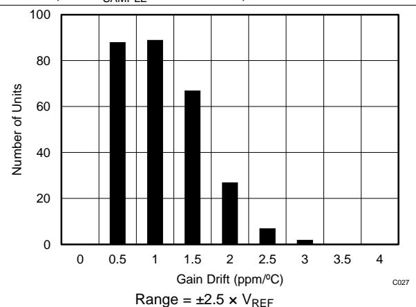
**Figure 27. Typical Histogram for Gain Error Drift**
