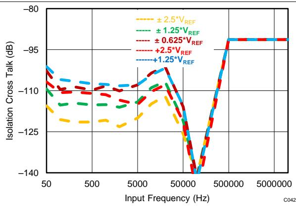
Figure 42. Isolation Crosstalk vs Frequency
