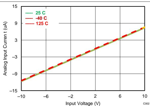
Figure 3. Input Current vs Temperature
