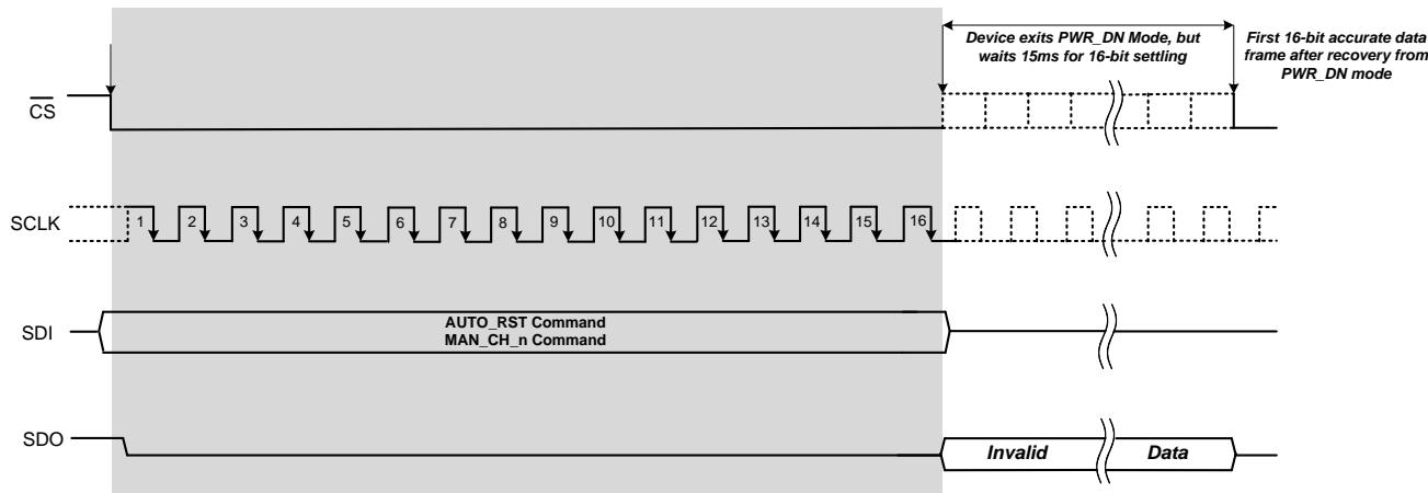
**Figure 80. Exit PWR\_DN Mode Timing Diagram**
