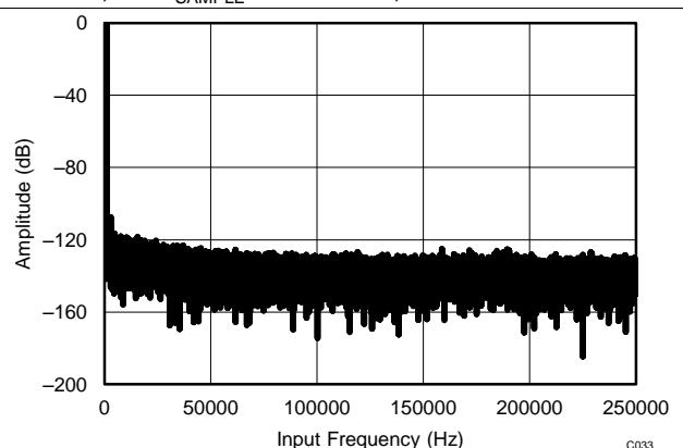
**Figure 33. Typical FFT Plot ( $2.5 \times V_{\text{REF}}$ )**
