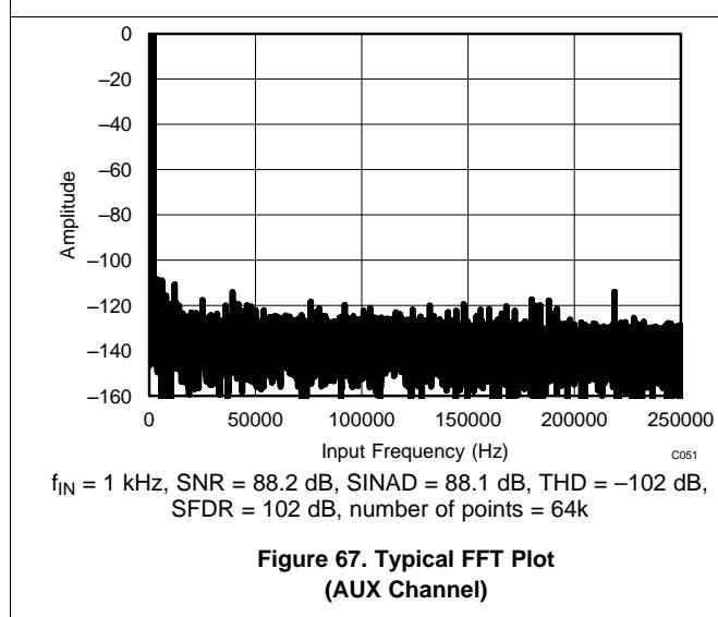
**Figure 67. Typical FFT Plot (AUX Channel)**
