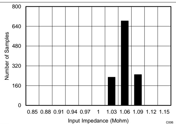
Figure 5. Typical Distribution of Input Impedance
