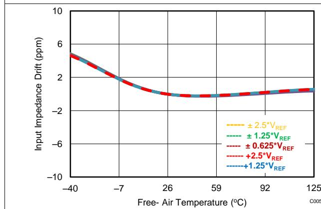
Figure 4. Input Impedance Variation vs Temperature
