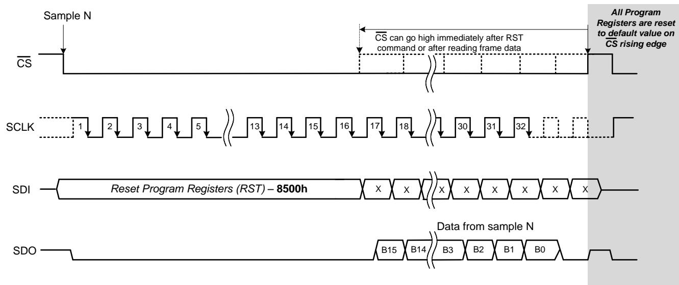
**Figure 87. Reset Program Registers (RST) Timing Diagram**
