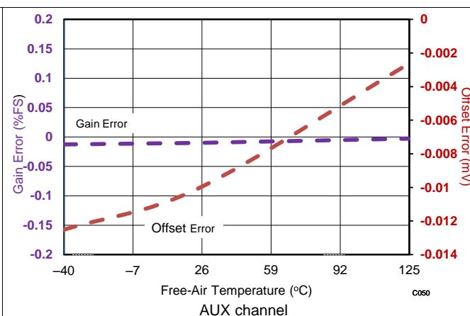
**Figure 66. Offset and Gain vs Temperature (AUX Channel)**
