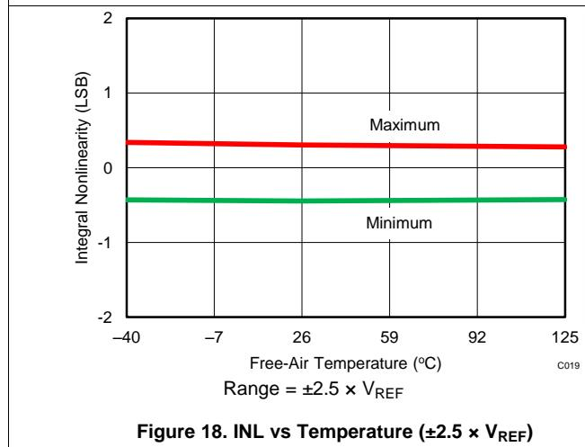
**Figure 18. INL vs Temperature ( $\pm 2.5 \times V_{\text{REF}}$ )**
