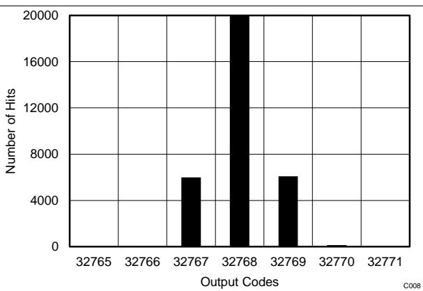
Figure 7. DC Histogram for Mid-Scale Inputs ( $\pm 1.25 \times V_{\text{REF}}$ )
