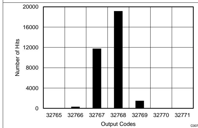
Figure 6. DC Histogram for Mid-Scale Inputs ( $\pm 2.5 \times V_{\text{REF}}$ )
