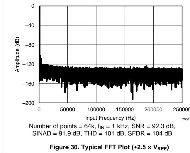
**Figure 30. Typical FFT Plot ( $\pm 2.5 \times V_{\text{REF}}$ )**
