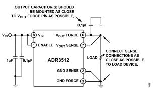
Figure 38. Application Showing Kelvin Connection
