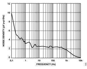
Figure 20. ADR3550 Output Noise Spectral Density
