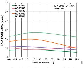
Figure 8. Load Regulation vs. Temperature (Sinking)
