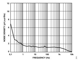
Figure 14. ADR3525 Output Noise Spectral Density
