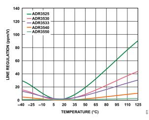
Figure 11. Line Regulation vs. Temperature
