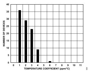
Figure 4. ADR3525 Temperature Coefficient Distribution
