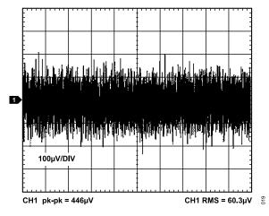
Figure 19. ADR3550 Output Voltage Noise (10 Hz to 10 kHz)
