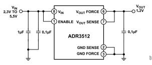
Figure 37. Basic Reference Connection
