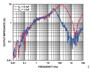
Figure 32. ADR3550 Output Impedance vs. Frequency
