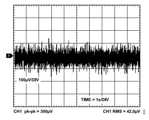
Figure 13. ADR3525 Output Voltage Noise (10 Hz to 10 kHz)
