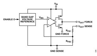
Figure 36. Block Diagram
