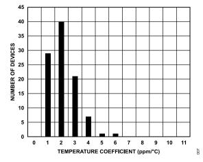
Figure 7. ADR3550 Temperature Coefficient Distribution
