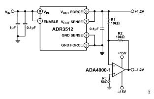
Figure 40. Bipolar Output Reference
