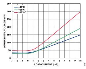
Figure 10. ADR3550 Dropout Voltage vs. Load Current
