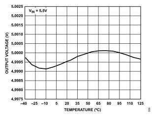
Figure 6. ADR3550 Output Voltage vs. Temperature
