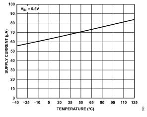
Figure 30. Supply Current vs. Temperature
