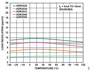
Figure 5. Load Regulation vs. Temperature (Sourcing)
