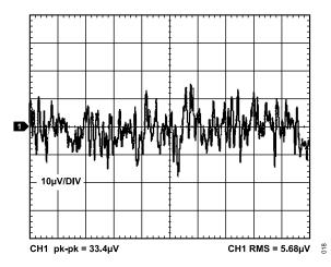
Figure 18. ADR3550 Output Voltage Noise (0.1 Hz to 10 Hz)
