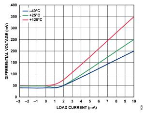
Figure 9. ADR3525 Dropout Voltage vs. Load Current
