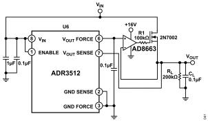
Figure 41. Boosted Output Current Reference
