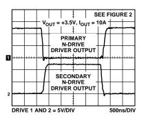
Figure 7. Gate Switching Waveforms
