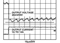
*Figure 10. Transient Response,* 1A–14 A of Figure 2 Circuit
