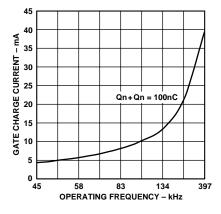
*Figure 6. Gate Charge vs. Supply Current*
