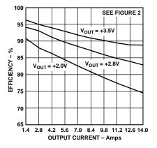
Figure 4. Efficiency vs. Output Current
