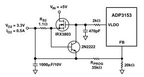
Figure 14. Linear Regulator with Overcurrent Protection
