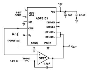
Figure 13. Closed-Loop Test Circuit for Accuracy
