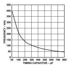
Figure 5. Frequency vs. Timing Capacitor
