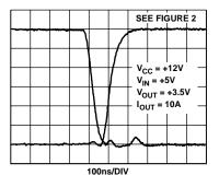
Figure 8. Driver Transition Waveforms
