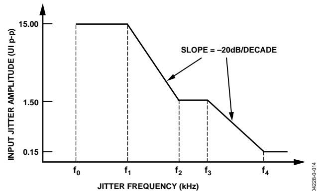
Figure 16. SONET Jitter Tolerance Mask
