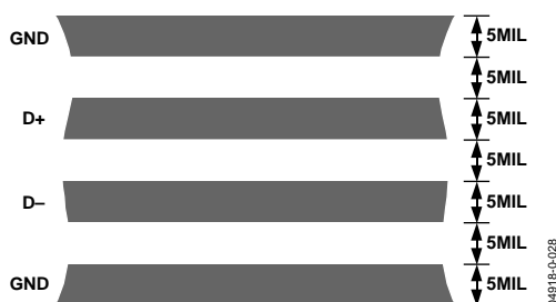
Figure 29. Arrangement of Signal Tracks
