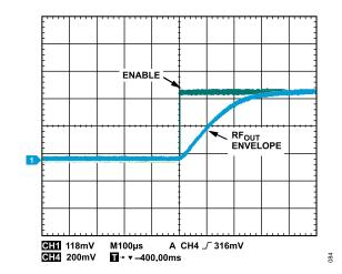
Figure 81. Turn-On Response Time of the RF Output (RF<sub>OUT</sub>) Envelope When IN Pin of the ADG719 Is Pulsed
