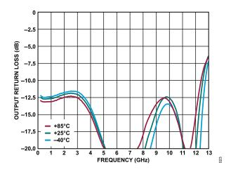
Figure 23. Output Return Loss vs. Frequency for Various Temperatures, 200 MHz to 13 GHz, V<sub>DD</sub> = 5 V, I<sub>DO</sub> = 95 mA
