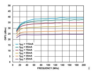
Figure 63. OIP3 vs. Frequency for Various  $I_{DQ}$  Values, 10 MHz to 200 MHz,  $V_{DD}$  = 5 V
