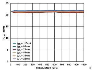
Figure 49.  $P_{SAT}$  vs. Frequency for Various I<sub>DQ</sub> Values, 10 MHz to 1000 MHz,  $V_{DD}$  = 5 V
