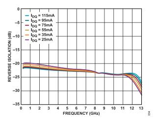
Figure 34. Reverse Isolation vs. Frequency for Various  $I_{DQ}$  Values, 200 MHz to 13 GHz,  $V_{DD}$  = 5 V
