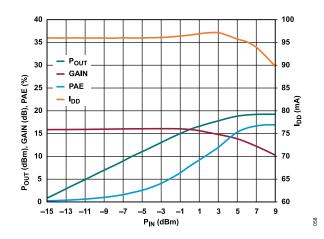
Figure 58. P<sub>OUT</sub>, Gain, PAE, and I<sub>DD</sub> vs. P<sub>IN</sub> at 11 GHz,  $R_{\rm BIAS}$  = 324  $\Omega$
