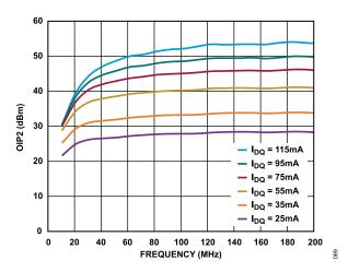
Figure 69. OIP2 vs. Frequency for Various  $I_{DQ}$  Values, 10 MHz to 200 MHz,  $V_{DD}$  = 5 V
