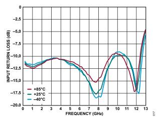
Figure 17. Input Return Loss vs. Frequency for Various Temperatures, 200 MHz to 13 GHz,  $V_{DD}$  = 5 V,  $I_{DQ}$  = 95 mA
