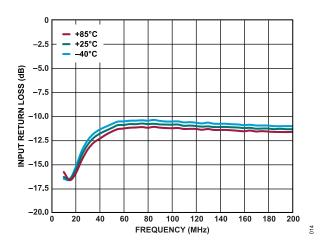
Figure 14. Input Return Loss vs. Frequency for Various Temperatures, 10 MHz to 200 MHz,  $V_{DD}$  = 5 V,  $I_{DQ}$  = 95 mA
