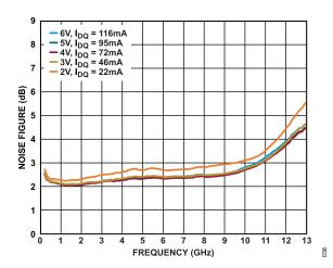
Figure 36. Noise Figure vs. Frequency for Various Supply Voltages and  $I_{DQ}$ Values, 200 MHz to 13 GHz,  $R_{BIAS}$  = 324  $\Omega$
