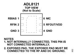
Figure 2. Pin Configuration
