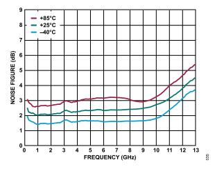
Figure 35. Noise Figure vs. Frequency for Various Temperatures, 200 MHz to 13 GHz,  $V_{DD}$  = 5 V,  $I_{DQ}$  = 95 mA
