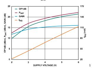
Figure 57. OP1dB, P<sub>SAT</sub>, Gain, and I<sub>DQ</sub> vs. Supply Voltage, at 8 GHz,  $R_{BIAS}$  = 324  $\Omega$
