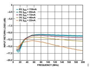
Figure 15. Input Return Loss vs. Frequency for Various Supply Voltages and  $I_{DQ}$  Values, 10 MHz to 200 MHz,  $R_{BIAS}$  = 324  $\Omega$
