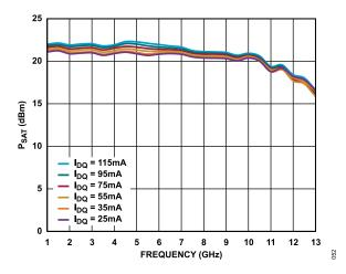
Figure 52.  $P_{SAT}$  vs. Frequency for Various  $I_{DQ}$  Values, 1 GHz to 13 GHz,  $V_{DD}$  = 5 V
