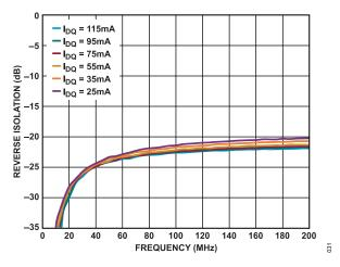
Figure 31. Reverse Isolation vs. Frequency for Various  $I_{DQ}$  Values, 10 MHz to 200 MHz,  $V_{DD}$  = 5 V
