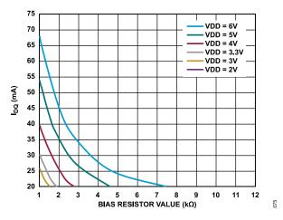
Figure 76.  $I_{DQ}$  vs. Bias Resistor Value, 1 k $\Omega$  to 12 k $\Omega$ , Various Supply Voltages
