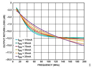
Figure 25. Output Return Loss vs. Frequency for Various  $I_{DQ}$  Values, 10 MHz to 200 MHz,  $V_{DD}$  = 5 V
