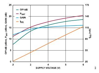
Figure 60. OP1dB, P<sub>SAT</sub>, Gain, and I<sub>DQ</sub> vs. Supply Voltage at 11 GHz,  $R_{BIAS}$  = 324  $\Omega$
