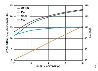
Figure 59. OP1dB,  $P_{SAT}$ , Gain, and  $I_{DQ}$  vs. Supply Voltage, at 5 GHz,  $R_{BIAS}$  = 324  $\Omega$
