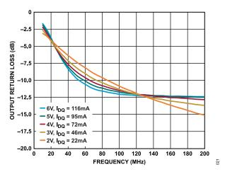
Figure 21. Output Return Loss vs. Frequency for Various Supply Voltages and  $I_{DQ}$  Values, 10 MHz to 200 MHz,  $R_{BIAS}$  = 324  $\Omega$
