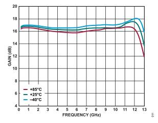
Figure 11. Gain vs. Frequency for Various Temperatures, 200 MHz to 13 GHz,  $V_{DD}$  = 5 V,  $I_{DQ}$  = 95 mA
