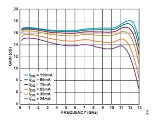
Figure 16. Gain vs. Frequency for Various  $I_{DQ}$  Values, 200 MHz to 13 GHz,  $V_{DD}$  = 5 V
