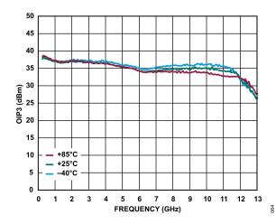
Figure 64. OIP3 vs. Frequency for Various Temperatures, 200 MHz to 13 GHz,  $V_{DD}$  = 5 V,  $I_{DQ}$  = 95 mA
