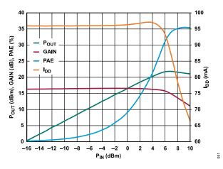
Figure 51. P<sub>OUT</sub>, Gain, PAE, and Drain Current (I<sub>DD</sub>) vs. Input Power (P<sub>IN</sub>) at 1 GHz, R<sub>BIAS</sub> = 324  $\Omega$
