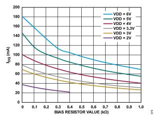
Figure 74. I<sub>DQ</sub> vs. Bias Resistor Value, 0 Ω to 1 kΩ, Various Supply Voltages
