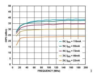
Figure 62. OIP3 vs. Frequency for Various Supply Voltages and I\_{DQ} Values, 10 MHz to 200 MHz, R\_{BIAS} = 324  $\Omega$
