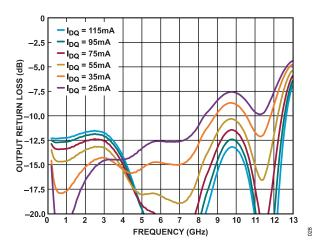
Figure 28. Output Return Loss vs. Frequency for Various I<sub>DQ</sub> Values, 200 MHz to 13 GHz, V<sub>DD</sub> = 5 V
