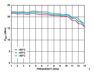
Figure 47.  $P_{SAT}$  vs. Frequency for Various Temperatures, 1 GHz to 13 GHz,  $V_{DD}$  = 5 V,  $I_{DQ}$  = 95 mA
