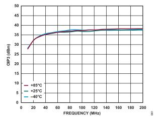
Figure 61. OIP3 vs. Frequency for Various Temperatures, 10 MHz to 200 MHz,  $V_{DD}$  = 5 V,  $I_{DQ}$  = 95 mA
