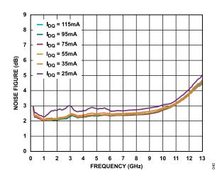
Figure 40. Noise Figure vs. Frequency for Various  $I_{DQ}$  Values, 200 MHz to 13 GHz,  $V_{DD}$  = 5 V
