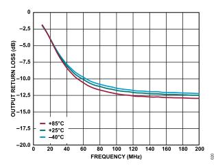
Figure 20. Output Return Loss vs. Frequency for Various Temperatures, 10 MHz to 200 MHz,  $V_{DD}$  = 5 V,  $I_{DQ}$  = 95 mA
