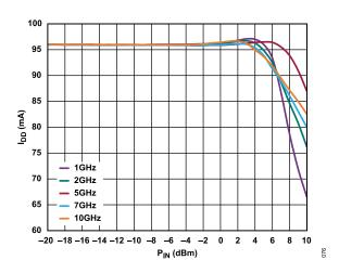
Figure 75.  $I_{DD}$  vs.  $P_{IN}$  for Various Frequencies,  $V_{DD}$  = 5 V
