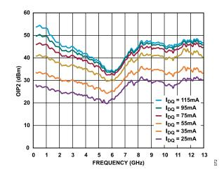
Figure 72. OIP2 vs. Frequency for Various I<sub>DQ</sub> Values, 200 MHz to 13 GHz,  $V_{DD}$  = 5 V
