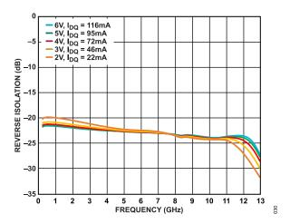
Figure 30. Reverse Isolation vs. Frequency for Various Supply Voltages and  $I_{DQ}$  Values, 200 MHz to 13 GHz,  $R_{BIAS}$  = 324  $\Omega$
