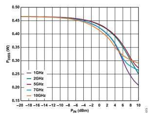
Figure 73.  $P_{DISS}$  vs.  $P_{IN}$  for Various Frequencies at 85°C,  $V_{DD}$  = 5 V,  $I_{DQ}$  = 95 mA
