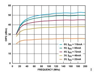
Figure 68. OIP2 vs. Frequency for Various Supply Voltages and I\_{DQ} Values, 10 MHz to 200 MHz, R\_{BIAS} = 324  $\Omega$
