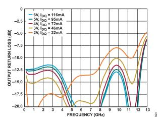
Figure 24. Output Return Loss vs. Frequency for Various Supply Voltages and I<sub>DQ</sub> Values, 200 MHz to 13 GHz,  $R_{BIAS}$  = 324  $\Omega$
