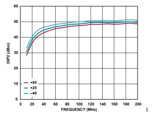
Figure 67. OIP2 vs. Frequency for Various Temperatures, 10 MHz to 200 MHz,  $V_{DD}$  = 5 V,  $I_{DQ}$  = 95 mA
