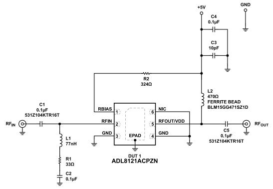
Figure 78. Typical Application Circuit
