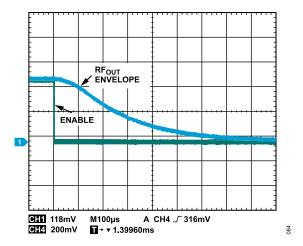
Figure 82. Turn-Off Response Time of the RF<sub>OUT</sub> Envelope When IN Pin of the ADG719 Is Pulsed
