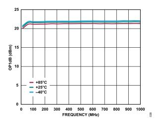
Figure 38. OP1dB vs. Frequency for Various Temperatures, 10 MHz to 1000 MHz, V<sub>DD</sub> = 5 V, I<sub>DQ</sub> = 95 mA
