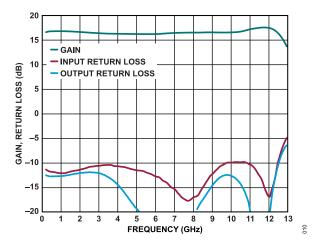
Figure 10. Gain and Return Loss vs. Frequency, 200 MHz to 13 GHz,  $V_{DD}$  = 5 V,  $I_{DQ}$  = 95 mA
