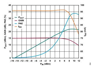
Figure 54.  $P_{OUT}$ , Gain, PAE, and  $I_{DD}$  vs.  $P_{IN}$  at 5 GHz,  $R_{BIAS}$  = 324  $\Omega$
