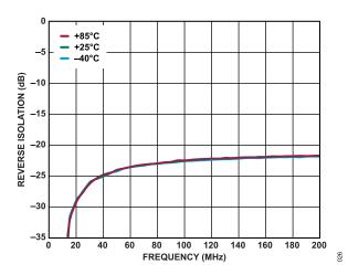
Figure 26. Reverse Isolation vs. Frequency for Various Temperatures, 10 MHz to 200 MHz,  $V_{DD}$  = 5 V,  $I_{DO}$  = 95 mA
