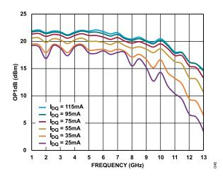
Figure 46. OP1dB vs. Frequency for Various  $I_{DQ}$  Values, 1 GHz to 13 GHz,  $V_{DD}$  = 5 V
