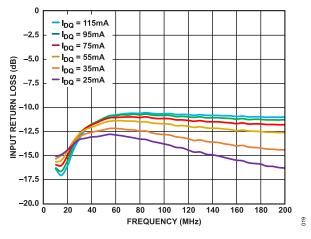
Figure 19. Input Return Loss vs. Frequency for Various I<sub>DQ</sub> Values, 10 MHz to 200 MHz, V<sub>DD</sub> = 5 V
