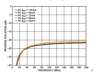
Figure 27. Reverse Isolation vs. Frequency for Various Supply Voltages and  $I_{DQ}$  Values, 10 MHz to 200 MHz,  $R_{BIAS}$ = 324  $\Omega$
