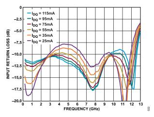
Figure 22. Input Return Loss vs. Frequency for Various  $I_{DQ}$  Values, 200 MHz to 13 GHz,  $V_{DD}$  = 5 V
