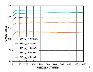
Figure 39. OP1dB vs. Frequency for Various Supply Voltages and I<sub>DQ</sub> Values, 10 MHz to 1000 MHz, R<sub>BIAS</sub> = 324  $\Omega$
