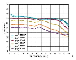
Figure 66. OIP3 vs. Frequency for Various I<sub>DQ</sub> Values, 200 MHz to 13 GHz,  $V_{DD}$  = 5 V
