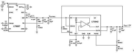
Figure 79. Recommended Power Management Circuit
