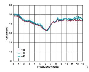
Figure 70. OIP2 vs. Frequency for Various Temperatures, 200 MHz to 13 GHz,  $V_{DD}$  = 5 V,  $I_{DQ}$  = 95 mA
