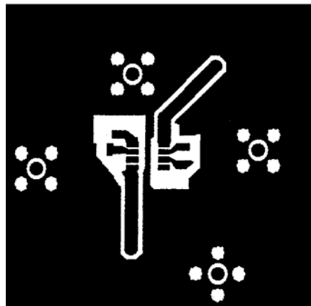
Figure 69. Noninverter SOIC Board Layout (Solder Side) (Looking Through the Board)
