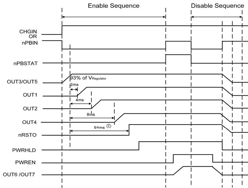
Ⓣ: Typical value shown, actual delay time may vary from (T-1ms) x 88% to T x 112%, where T is the typical delay time setting.
