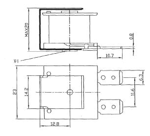
Dimensions: Millimetres Tolerance: ±0.5mm
