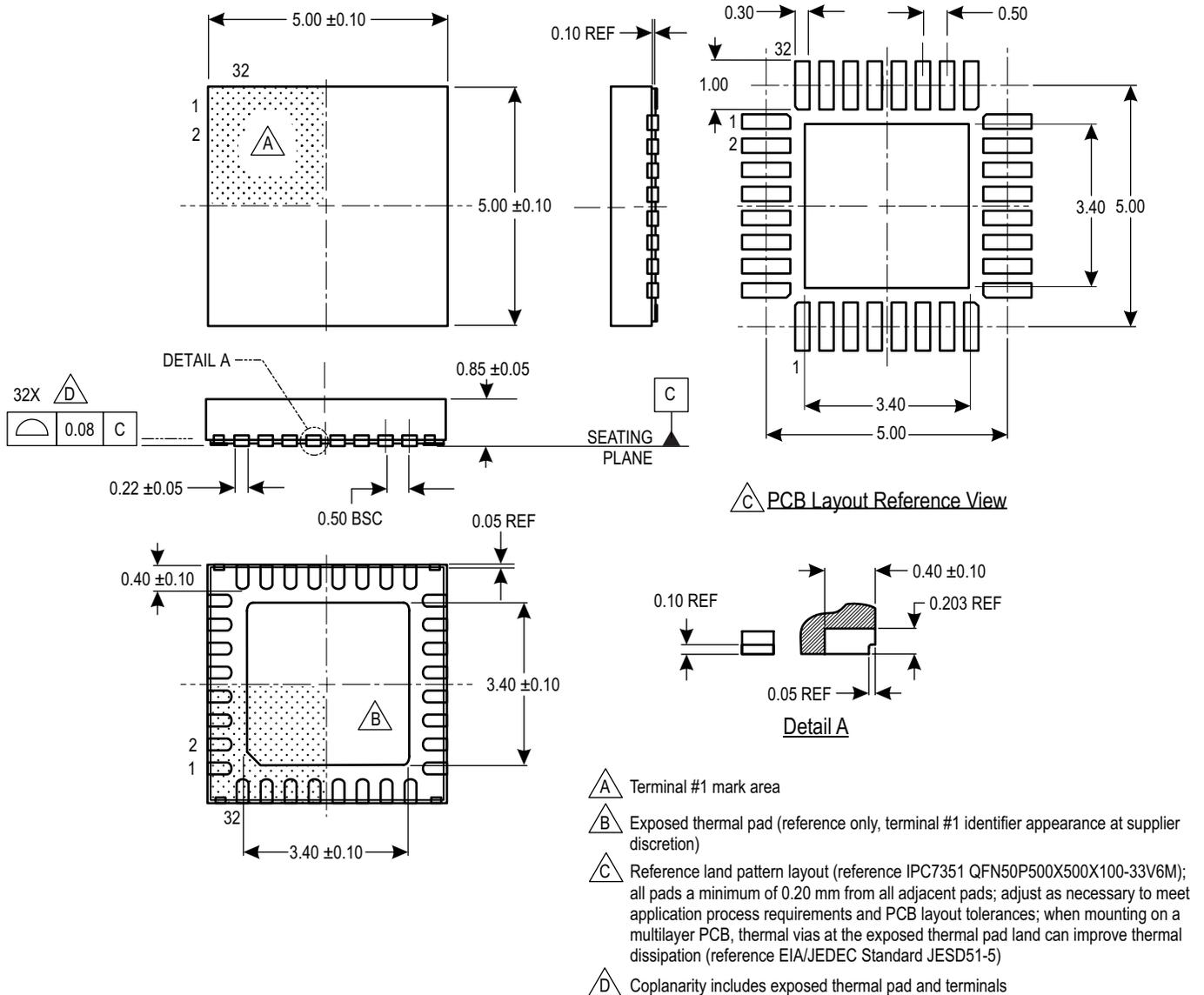
**Figure 31: 32-Pin 5 mm × 5 mm QFN with exposed thermal pad and wettable flank (suffix ET)**
