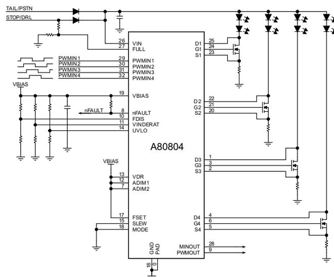
Figure 1: Typical Application Diagram with External PWM
