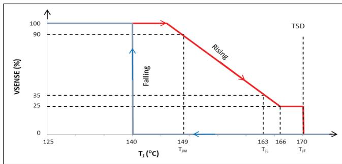
**Figure 20: Output Current Foldback Based on Rising  $T_J$**
