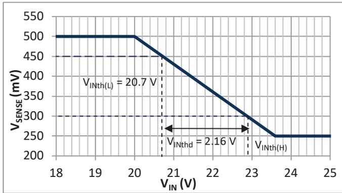
**Figure 19: Output Current Foldback Based on  $V_{IN}$**
