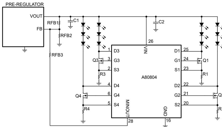
**Figure 9: Example of Using MINOUT with Pre-regulator**
