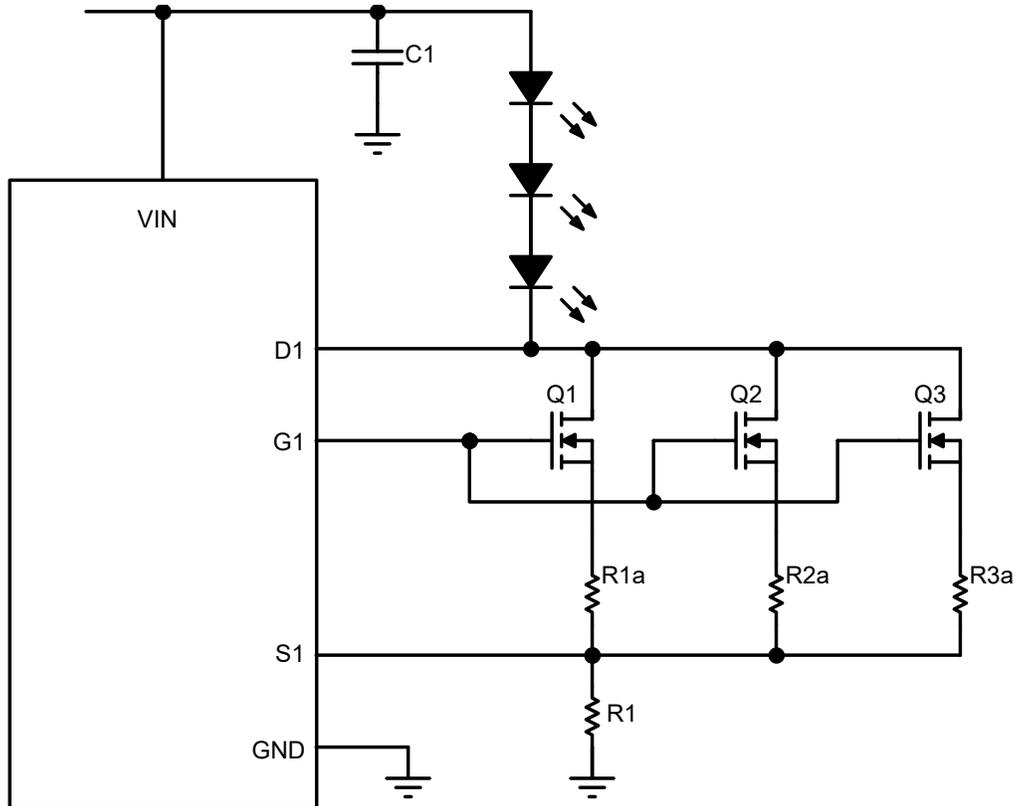
Figure 29: Parallel MOSFET Arrangement for High Power Application
