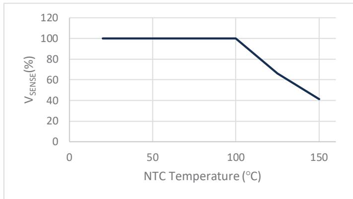
**Figure 28: Typical External Thermal Derating and Binning Arrangement**
