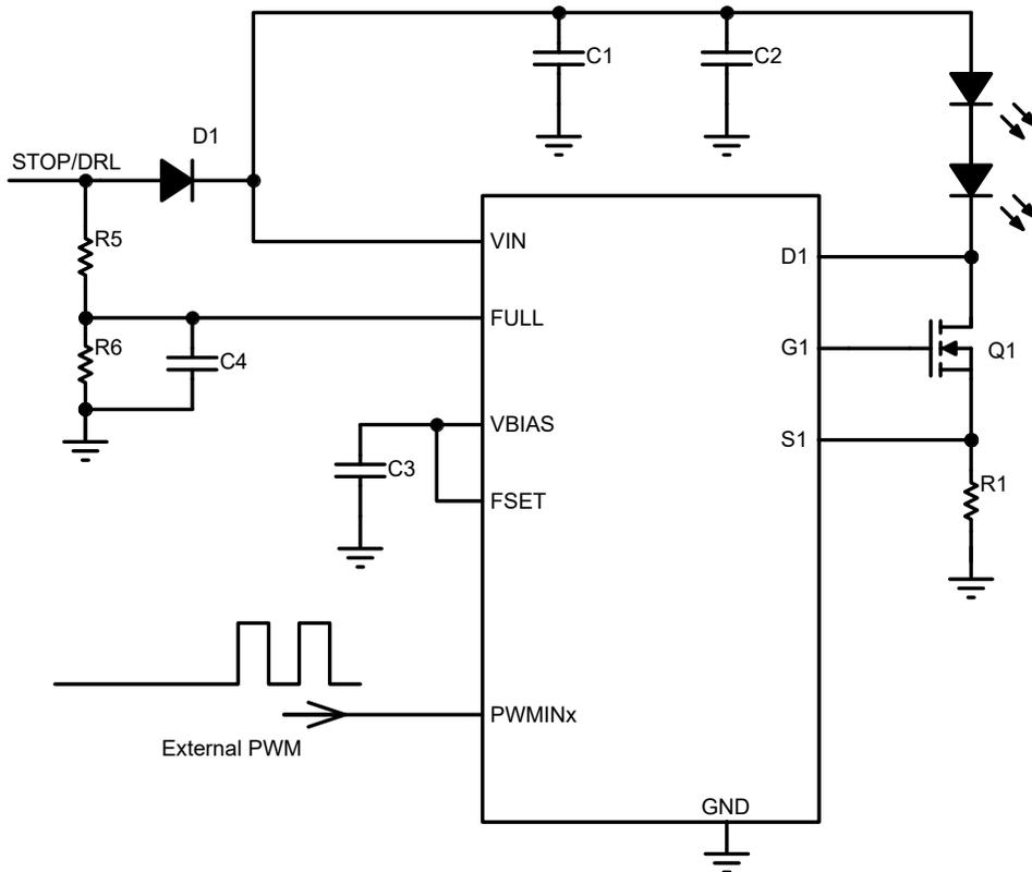
**Figure 30: Application to avoid initial LED current in external PWM mode with FULL pin connected to VIN and PwMINx held low at startup.**
