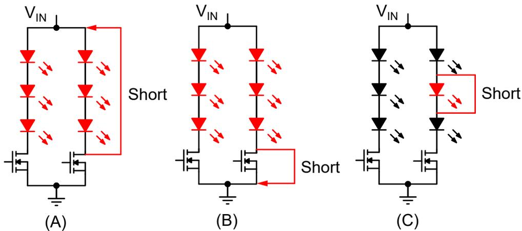
**Figure 14: Short-Circuit Protection**
