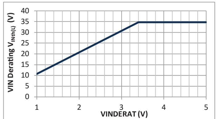
**Figure 18:  $V_{VINDERAT}$  Voltage versus  $V_{IN}$  Derating Threshold**
