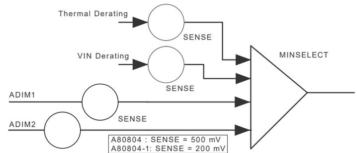
**Figure 22: Analog Dimming and Derating Block Diagram**
