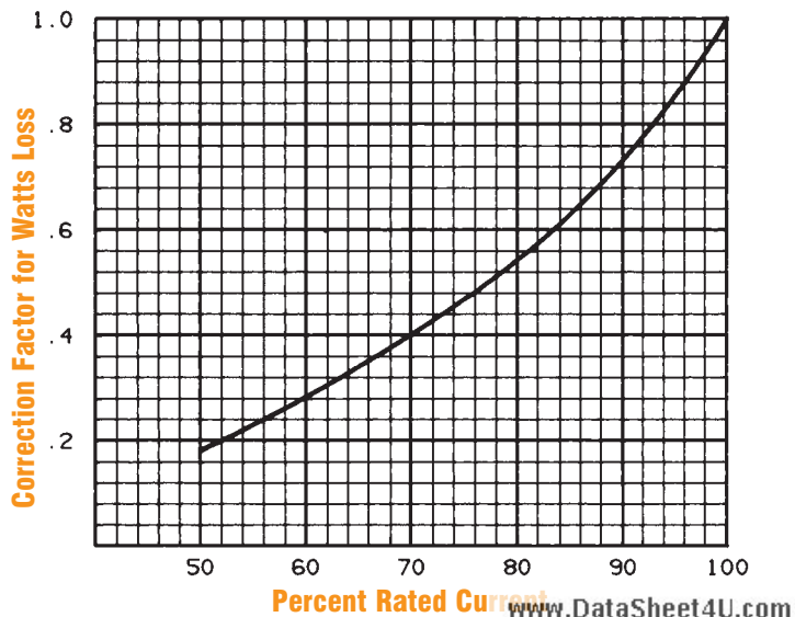
Watts Loss vs. % Rated Current
