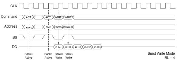
WRITE to WRITE Command Interval (different bank)
