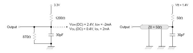
(Fig. 1) DC output load circuit
