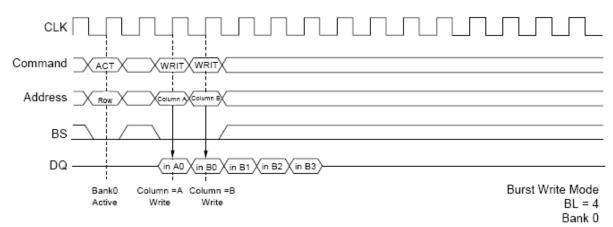
WRITE to WRITE Command Interval (same ROW address in same bank)
