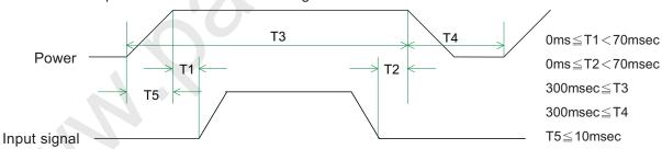
Apply the lamp voltage within the LCD operating range. When the backlight turns on before the LCD operation or the LCD turns off before the backlight turns off, the display may momentarily become abnormal.
