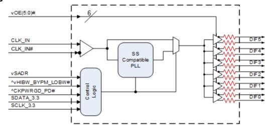
Note: Default resistors are internal on xx41/xx51 devices. P1 devices have programmable default impedances on an output-by-output basis.
