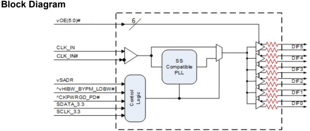
Note: Default resistors are internal on xx41/xx51 devices. P1 devices have programmable default impedances on an output-by-output basis.
