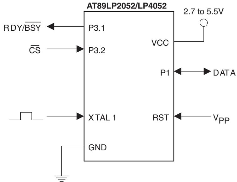
Note: Sampling of pin P3.1 (RDY/BSY) is optional. During Parallel Programming, P3.1 will be pulled low while the device is busy. Note that it does not require an external passive pull-up to  $V_{CC}$ .
