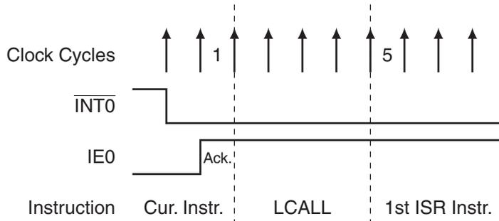
**Figure 13-2.** Maximum Interrupt Response Time
