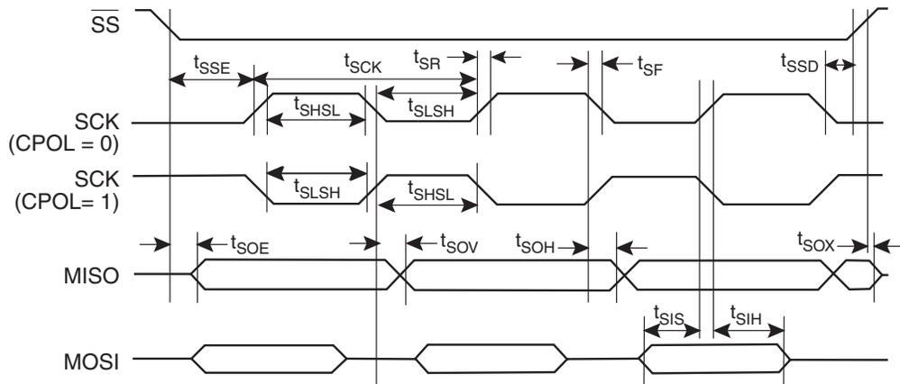
**Figure 23-3. SPI Master Timing (CPHA = 1)**
