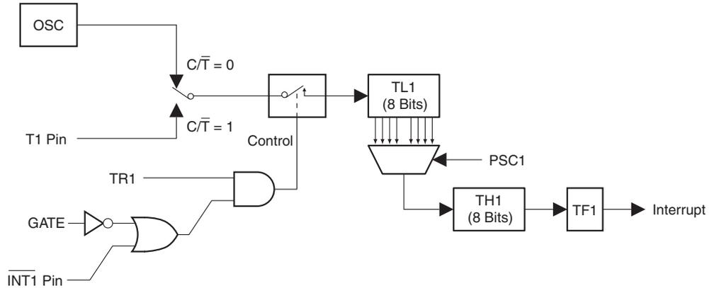
Mode 0 operation is the same for Timer 0 as for Timer 1, except that TR0, TF0 and  $\overline{\text{INT0}}$  replace the corresponding Timer 1 signals in [Figure 15-1](#). There are two different GATE bits, one for Timer 1 (TMOD.7) and one for Timer 0 (TMOD.3).
