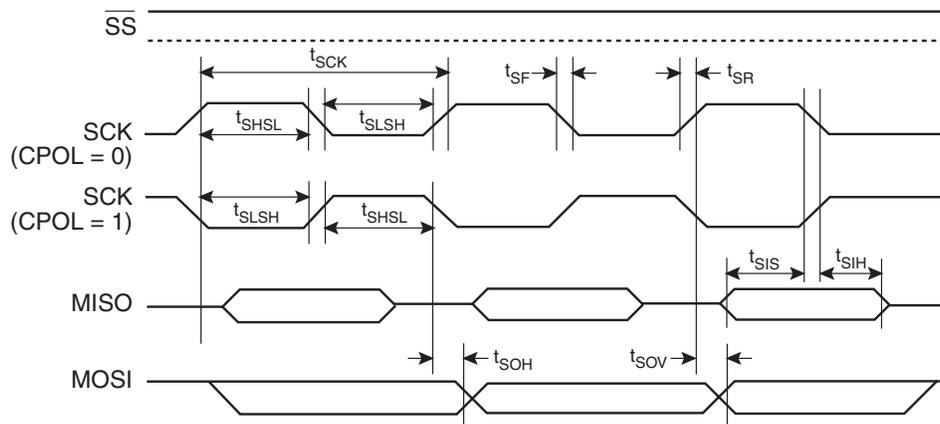
**Figure 23-4.** SPI Slave Timing (CPHA = 1)
