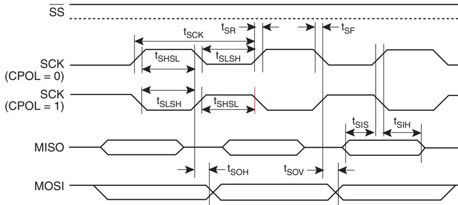
**Figure 23-2. SPI Slave Timing (CPHA = 0)**
