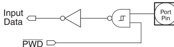
**Figure 14-3.** Input Only for P3.2 and P3.3
