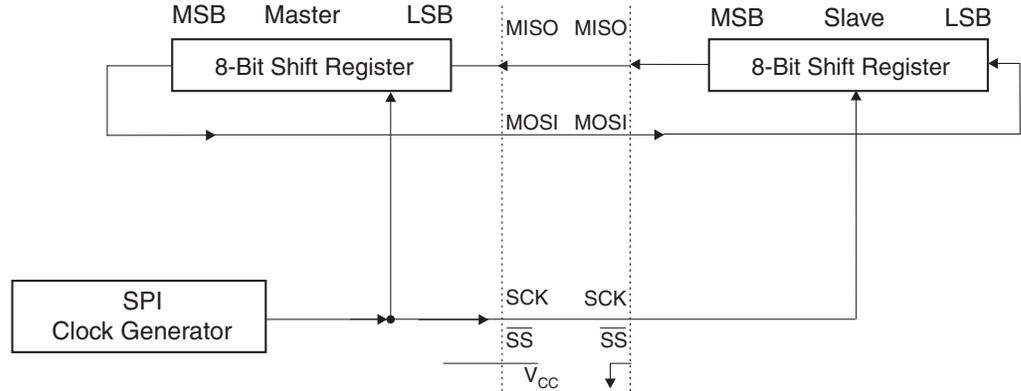
**Figure 18-2.** SPI Block Diagram
