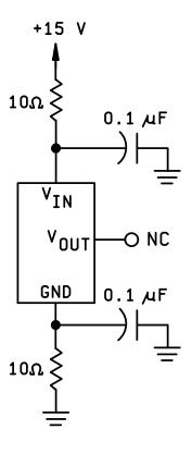
FIGURE 2. Radiation exposure circuit.
