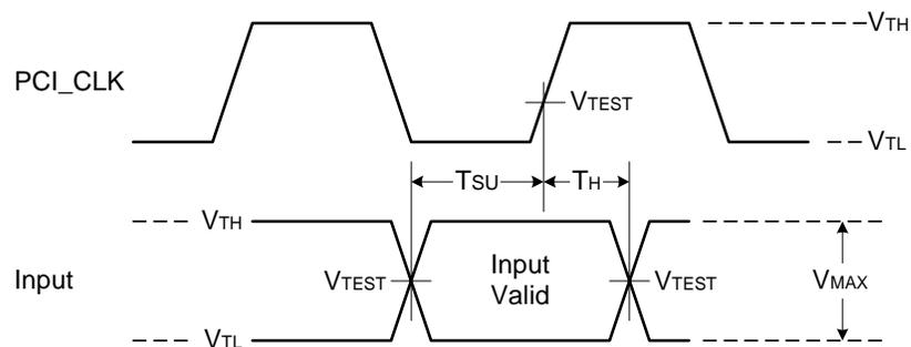
Table 16. PCI Bus Interface Timing Measurement Conditions
