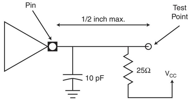
Figure 7. TVAL (min) Test Load
