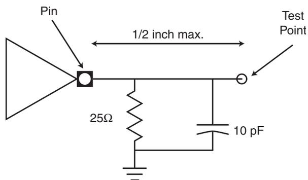
Figure 6. TVAL (max) Falling Edge Test Load
