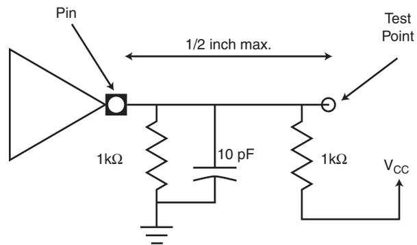
Figure 8. TVAL Test Load (PCI 5 V Signaling Environment)
