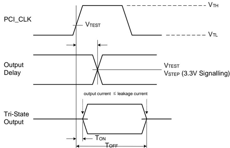
Figure 4. PCI Bus Interface Input Timing Measurement Conditions
