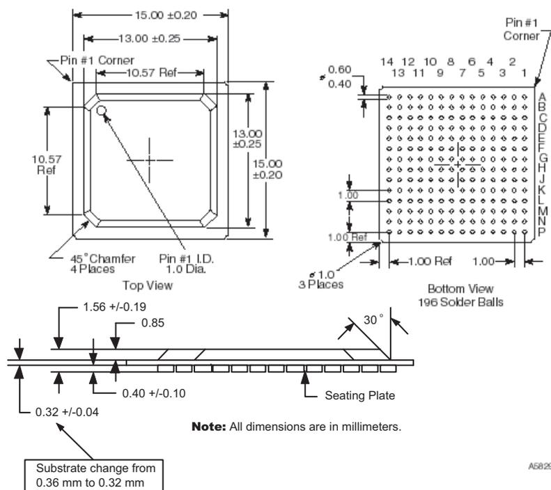
**Figure 11. Mechanical Specifications**
