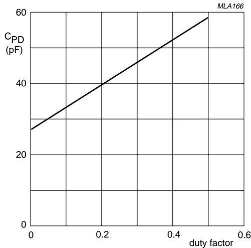
Fig.6 C<sub>PD</sub> as a function of the duty factor.**POWER DISSIPATION INFORMATION**
