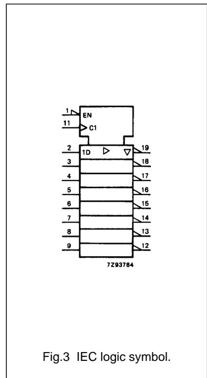
Octal D-type flip-flop; positive-edge trigger;
