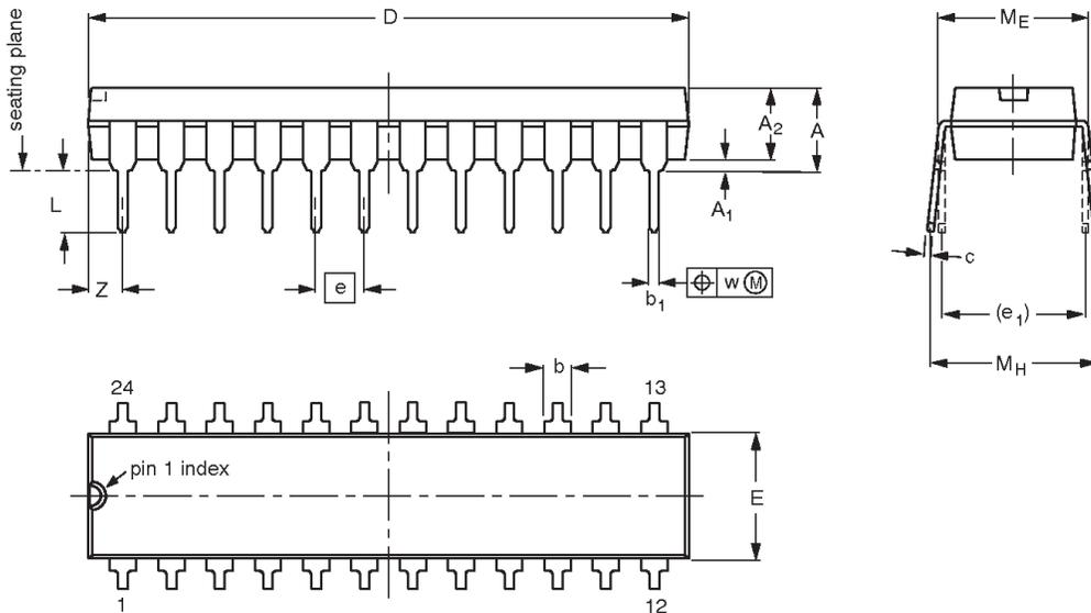
**DIMENSIONS (millimetre dimensions are derived from the original inch dimensions)**
