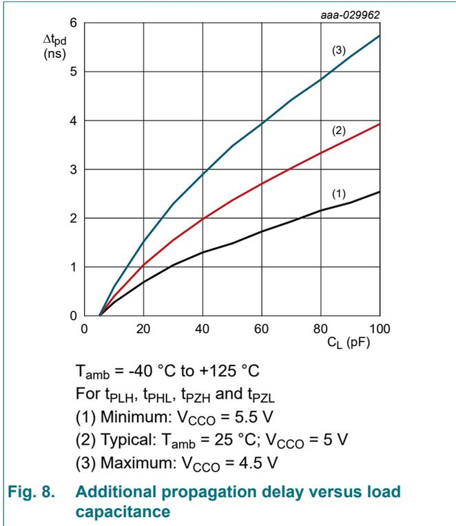
Fig. 8. Additional propagation delay versus load capacitance
