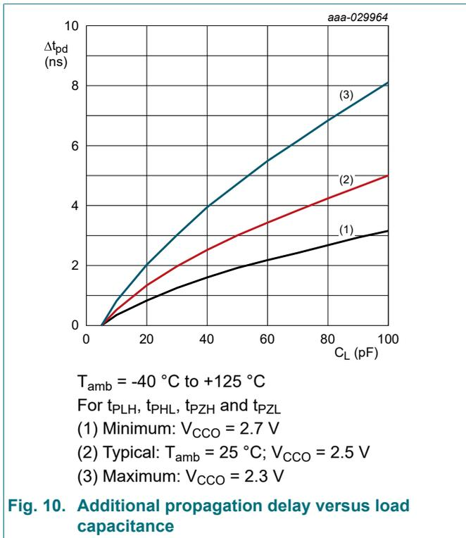
Fig. 10. Additional propagation delay versus load capacitance
