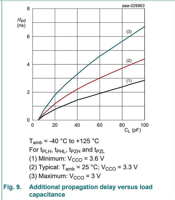
Fig. 9. Additional propagation delay versus load capacitance
