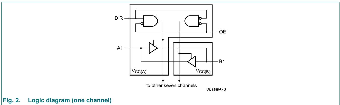
Fig. 2. Logic diagram (one channel)
