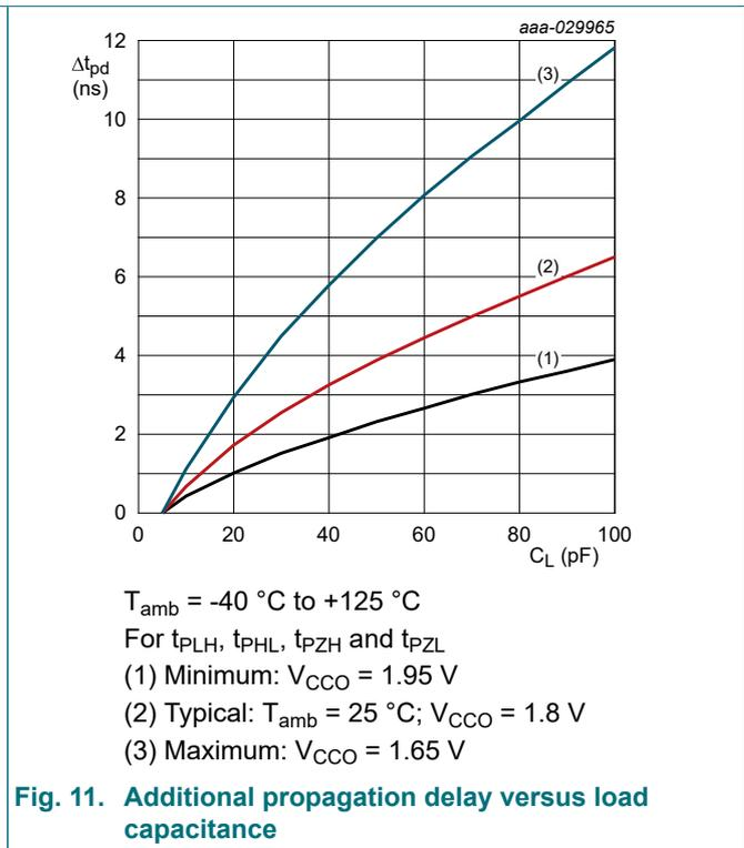
Fig. 11. Additional propagation delay versus load capacitance
